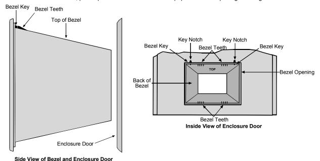
Figure 2: Installing the Viewing Bezel
