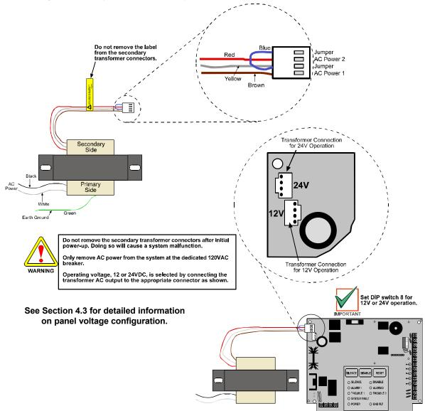
Figure 5: Connecting the Transformer to the D7022
