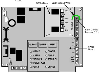
Figure 15: Locating the D7025 on the D7022
