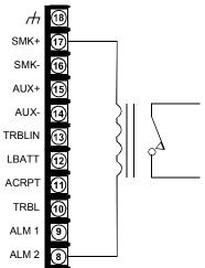
Use 12 V relays for 12 V configuration Use 24 V relays for 24 V configuration
