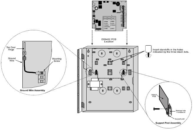
Figure 4: D7022 Control Panel Installation
