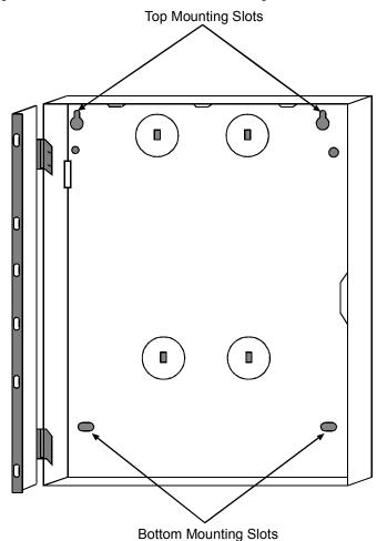
Figure 1: Mounting the Enclosure
