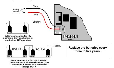
Figure 6: Battery Connections
