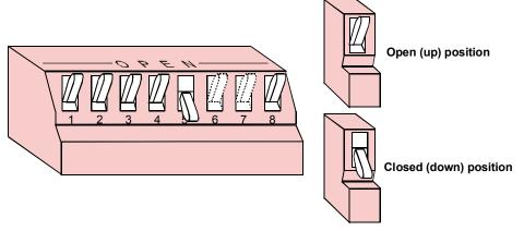
Figure 11: DIP Switch Orientation
