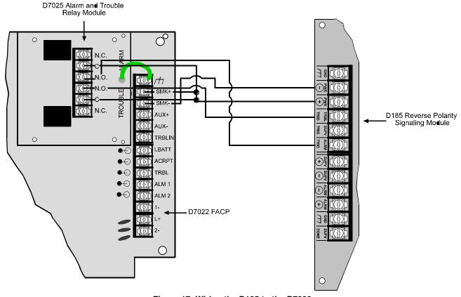
Figure 17: Wiring the D185 to the D7022
