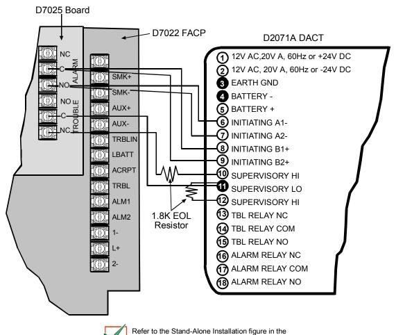
Figure 18: Wiring the D2071A to the D7022
