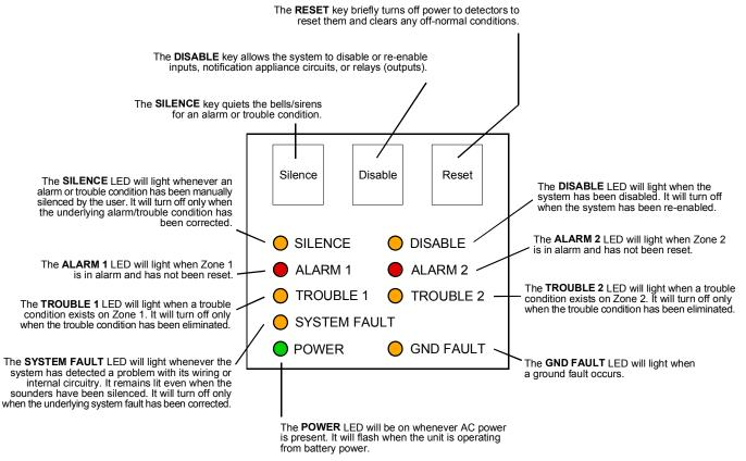
Figure 13: The D7022 Built-In Keypad
