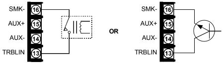
Figure 9: Typical Wiring for the Trouble Input
