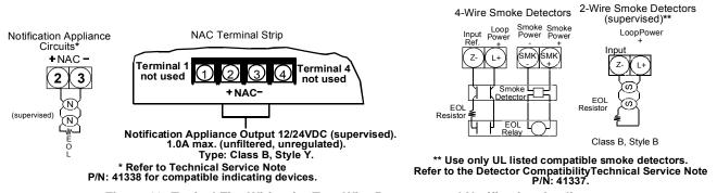
Figure 10: Typical Fire Wiring for Two-Wire Detectors and Notification Appliances
