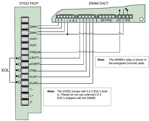
Figure 19: Wiring the D9068 to the D7022
