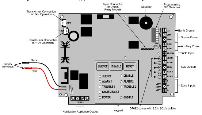
Figure 3: D7022 Control Panel
