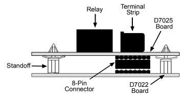
Figure 16: Connecting the D7025 to the D7022
